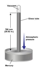
A mercury barometer is an instrument for measuring air pressure. Today, many meteorologists use new aneroid barometers. This is partly because mercury is toxic and partly because it is easier to take multiple measurements with aneroid barometers.
