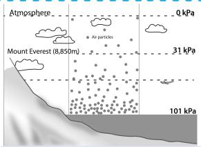
Particles of cool air sink, creating areas of high pressure. Particles of warm air rise, creating areas of low pressure. The air pressure at the top of Mount Everest (measured in kPa, or kilopascals) is more than three times lower than at Earth's surface.
